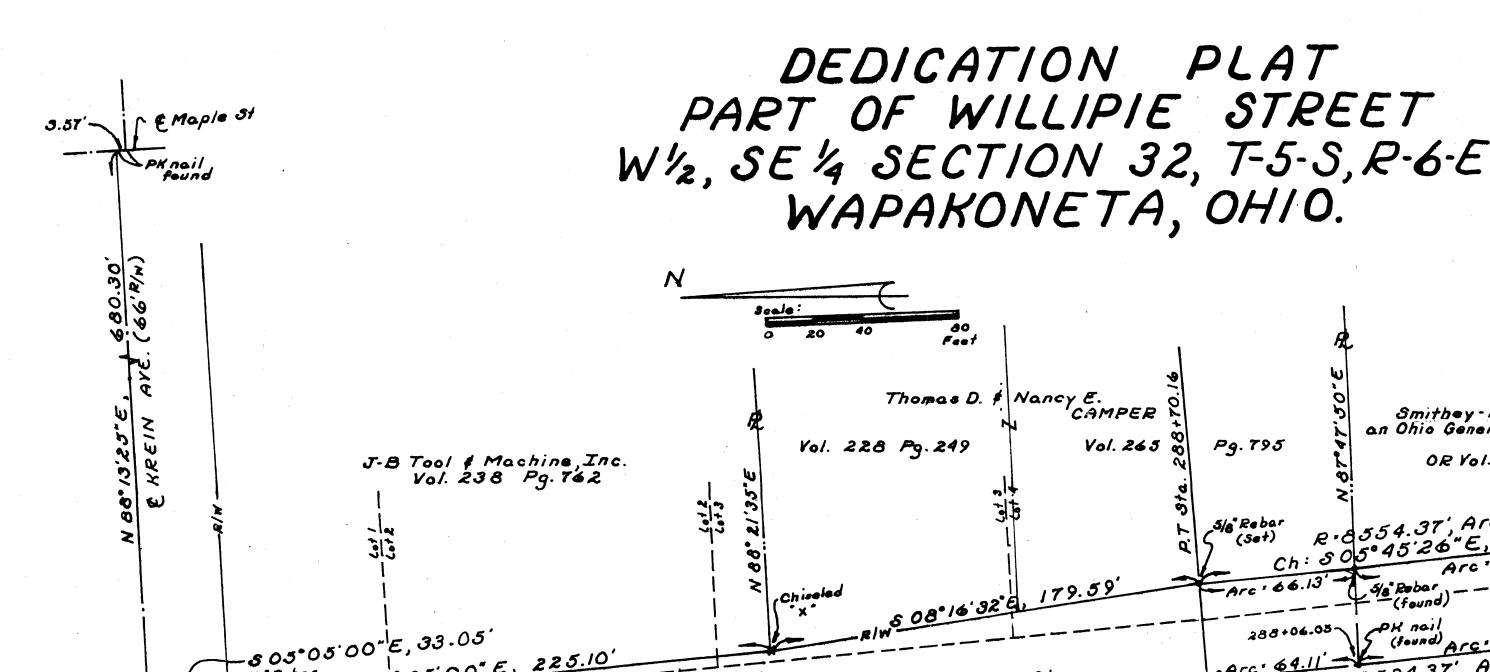
(Set) Ch: NO5. 44'50" W, 199.11' CENTERLINE CURVE DATA P.I. Sta. 287+22.12 △· /° 58′30″ T. 148.07 R.8594.37 L= 296.11'
