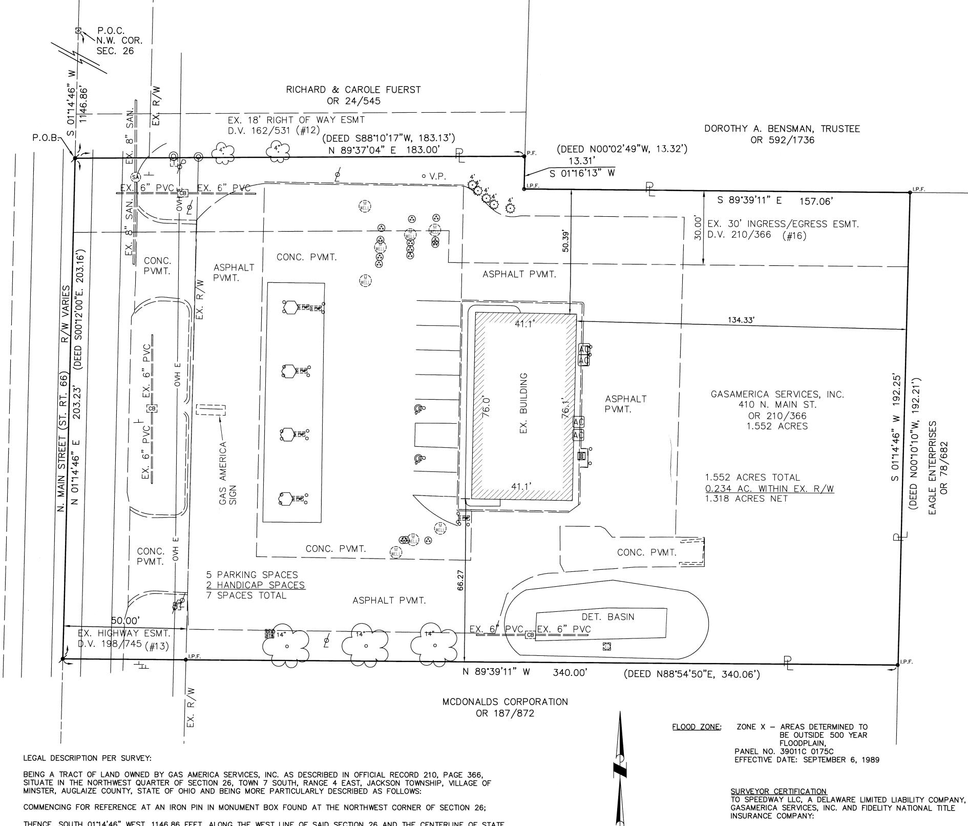
THENCE, SOUTH 01"14'46" WEST, 1146.86 FEET, ALONG THE WEST LINE OF SAID SECTION 26 AND THE CENTERLINE OF STATE ROUTE 66 TO A MAG NAIL SET AND BEING THE PRINCIPAL PLACE OF BEGINNING FOR THE TRACT HEREIN CONVEYED;
