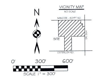
BASIS OF BEARING: BEARINGS ARE BASED UPON THE OHIO DEPARTMENT OF TRANSPORATION V.R.S., NAD 83(2011ADJ.) OHIO STATE PLANE NORTH ZONE 3401.
