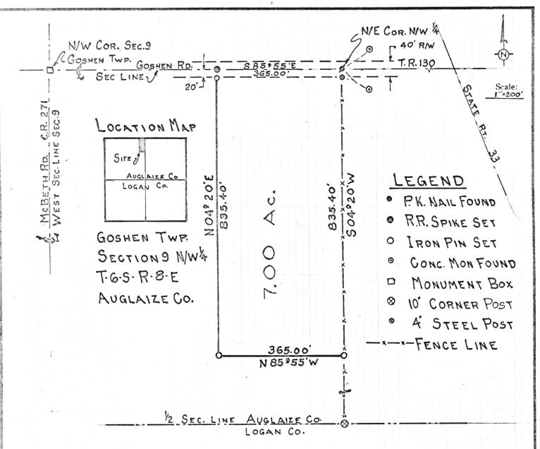
Being 7.00 Acres located in the north-west quarter of Section 9, T-6-S, R-8-E, Goshen Township, Auglaize County, Ohio and being further described as follows: Commencing at a P.K. nail and shiner found at the North-East corner of the North-West quarter of Section 9 and the PLACE OF BEGINNING.
