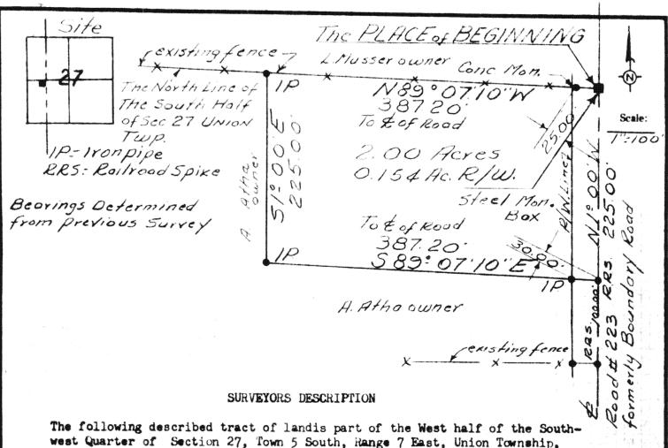
west Quarter of Section 27, Town 5 South, Range 7 East, Union Township, Auglaize County, Ohio, and is more particularly described as follows. The PLACE OF BEGINNING being a steel monument box over an iron pin at the intersection of the centerline of Road #223, formerly Boundary Road, and the North line of the South half of Section 27, Union Township.
