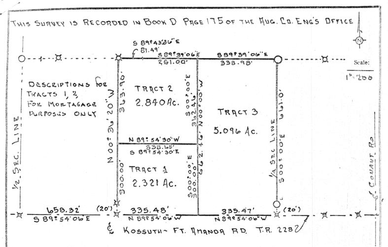
TRACTS ONE, TWO AND THREE ARE SPLITS OF ORIGINAL SURVEY CONDUCTED BY: THOMAS W. STEINKE & ASSOC. INC. DRAWING NO. 77-370 WHICH SURVEY IS RECORDED IN BOOK C PAGE LL OF THE AUGLAIZE COUNTY ENGINEERS OFFICE SURVEY RECORDS DRIGINAL SURVEY CONSISTED OF 10.257 ACRES.
