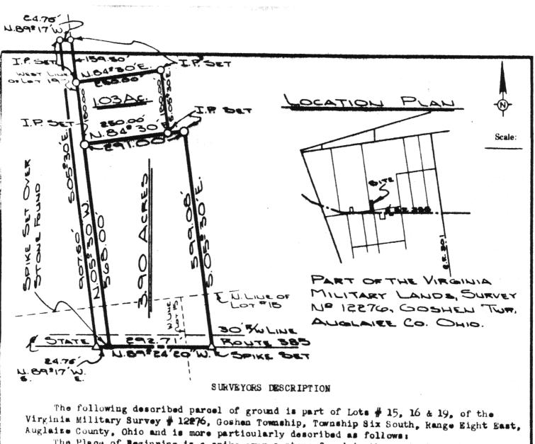
The Place of Beginning is a spike over a stone found in the centerline of State Route # 385 and the projected West line of Lot # 19 of the Virginia Military Survey # 12276; Thence NO5 -30 W a distance of 568.00 feet to an iron pin in the West line of said Lot # 19;
