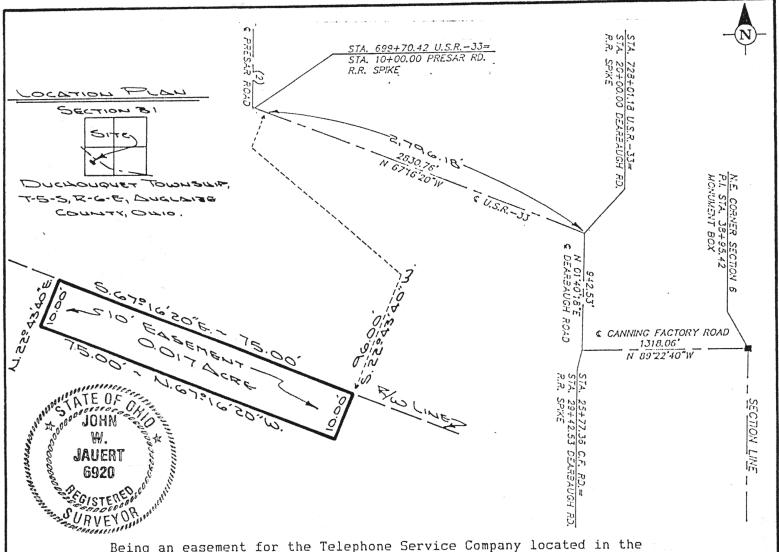
Being an easement for the Telephone Service Company located in the Southwest Quarter of Section 31, Town 5 South, Range 6 East, Duchouquet Township, Auglaize County, Ohio and being further described as follows:
