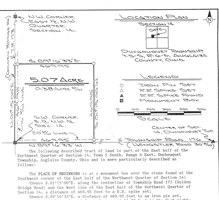
thence S.89°16'33"E. a distance of 469.95 feet to an iron pin set, passing thru an iron pin set for reference at 16.00 feet in the East right-of-way line of Township Road 173;
