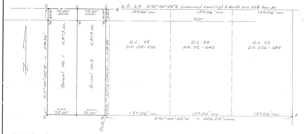
IEGEND A = Exist. 1/8" rod B = Set # 5 rebar C = Set PK nail
