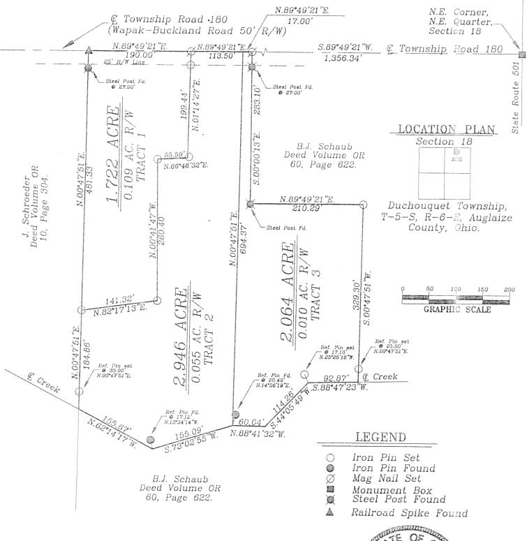
Basis of bearing is holding the North line of the Northeast Quarter of Section 18, and the centerline of Wapak—Buckland Road as N.89°49'21"E.
