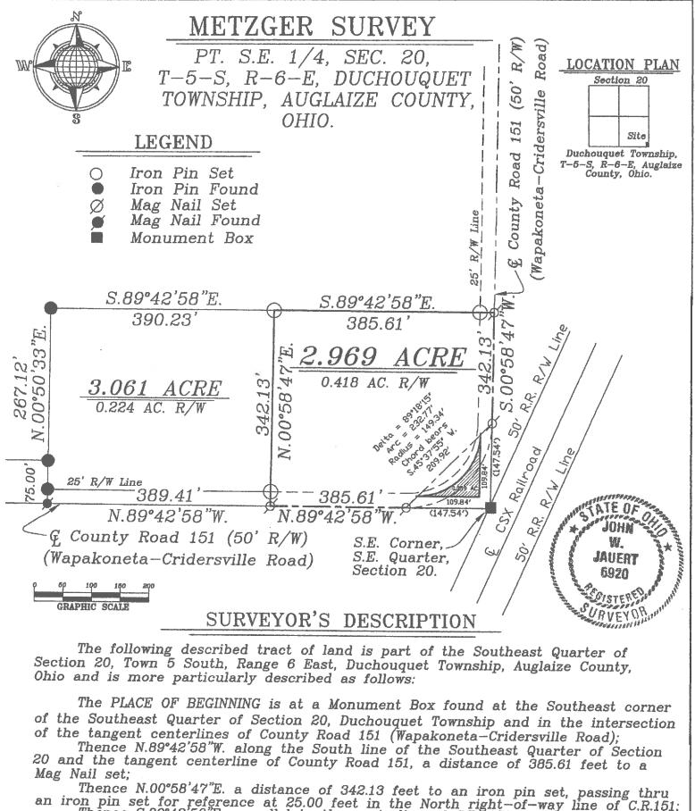
Thence N.00°58'47"E. a distance of 342.13 feet to an iron pin set, passing thru an iron pin set for reference at 25.00 feet in the North right-of-way line of C.R.151; Thence S.89°42'58"E., parallel to the centerline of C.R. 151 and the South line of the Southeast Quarter of Section 20, a distance of 385.61 feet to a Mag nail set, passing thru an iron pin set for reference at 360.61 feet in the West right-of-way line of County Road 151;
