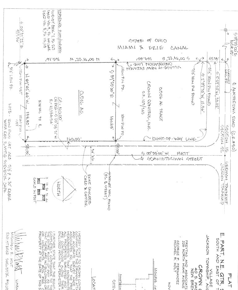
E. PART, N.E. QTR, SECTION 22, T 7 S, R 4 E, SOUTH AND EAST OF THE FIRST PRINCIPAL MERIDIAN IN THE VILLAGE OF NEW BREMEN JACKSON TOWNSHIP, AUGLAIZE COUNTY, STATE OF OHIO PLAT OF SURVEY
