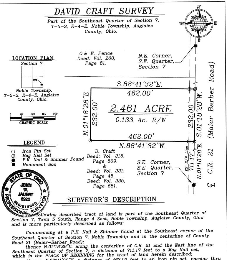
thence N.88°41'32"W. a distance of 462.00 feet to an iron pin set, passing thru an iron pin set for reference at 25.00 feet in the West right-of-way line of County Road 21;
