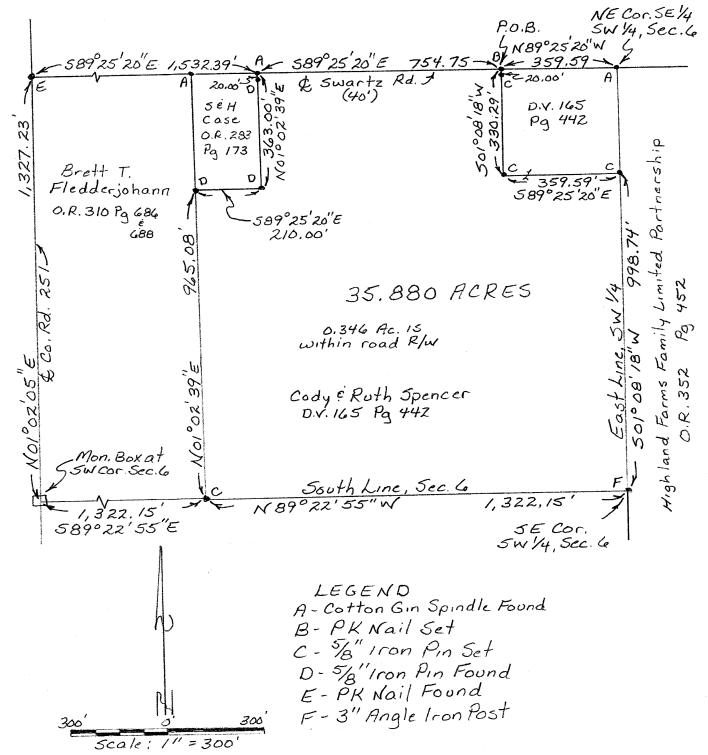
This plat represents an actual field survey performed in September, 2005. All markers are accurate as to materials and location and are in place. All bearings refer to the centerline of Swartz Road as being S 89° 25' 20" E
