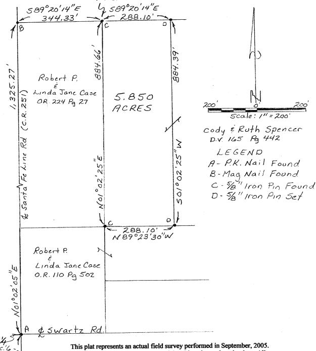
S.W. Cor. NW4 5W14, Sec. 6 All markers are accurate as to material and location and are in place. All bearings refer to the centerline of County Road 251 as being N 01° 02' 05" E
