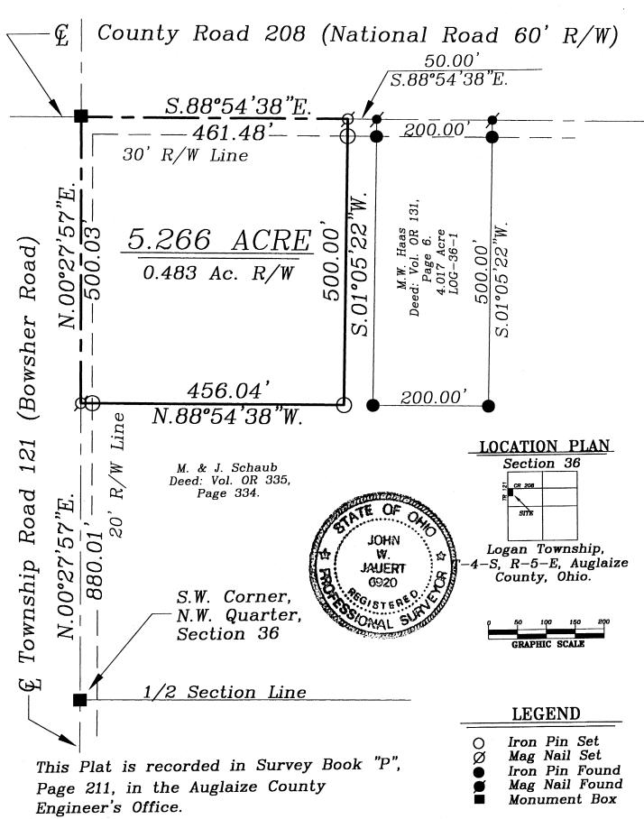
Bearing Basis: Centerline of T.R. 121 as N.00°27'57"E. Auglaize County GPS Data.
