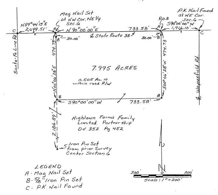
This plat represents an actual field survey performed in December, 2005. All markers are accurate as to material and location and are in place. All bearings refer to the centerline of State Route 33 as being N 90° 00' 00" E
