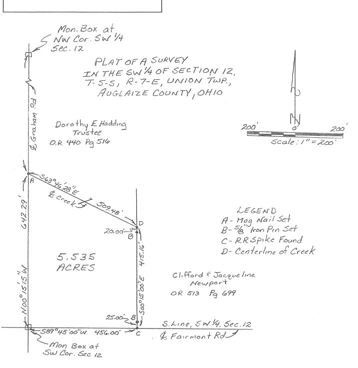
This plat represents an actual field survey performed in December, 2006. All markers are accurate as to material and location and are in place. All bearings refer to the South line of the Southwest Quarter of Section 12 as being S 89° 45' 00" W
