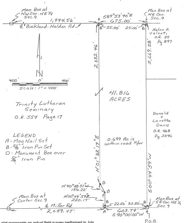
This plat represents an actual field survey performed in July, 2007. All markers are accurate as to material and location and are in place. All bearings refer to the centerline of Miller Road as being N 90° 00' 00" E
