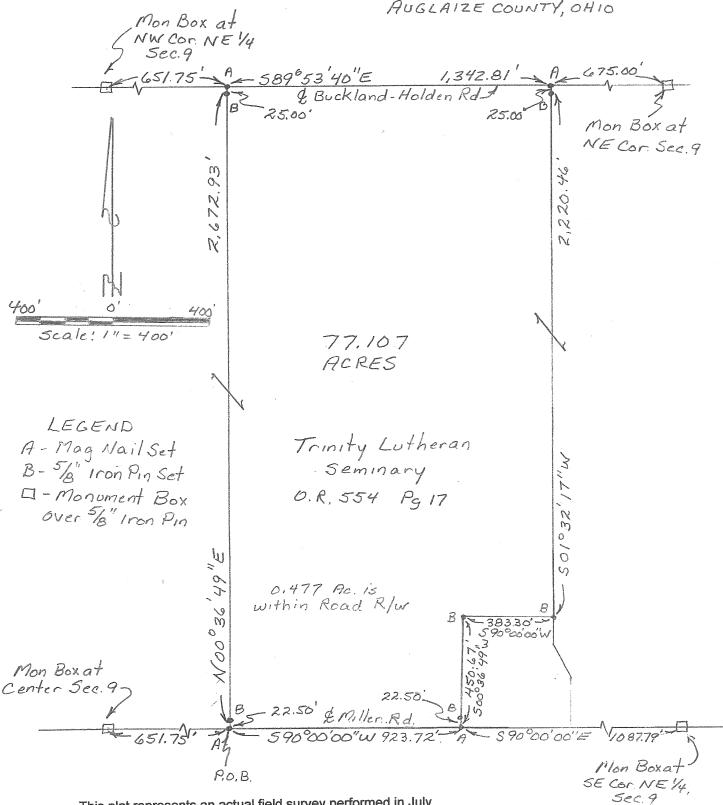
This plat represents an actual field survey performed in July, 2007. All markers are accurate as to material and location and are in place. All bearings refer to the centerline of Miller Road as being N 90° 00' 00" E
