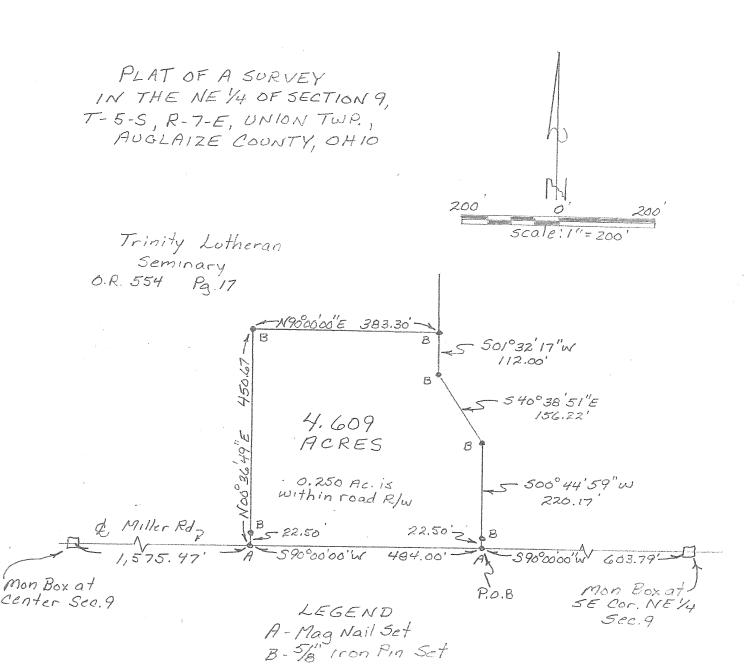
This plat represents an actual field survey performed in September, 2007. All markers are accurate as to material and location and are in place. All bearings refer to the centerline of Miller road as being S 90° 00' 00" W
