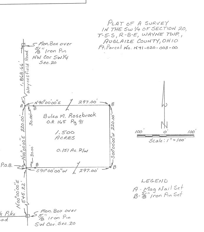
This plat represents an actual field survey performed in January, 2008. All markers are accurate as to material and location and are in place. All bearings refer to the centerline of Waynesfield Road as being N 00° 00' 00" E
