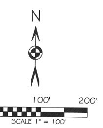
BASIS OF BEARING: BEARINGS SHOWN ARE ASSUMED AND SHOWN FOR ANGULAR MEASUREMENT ONLY.
