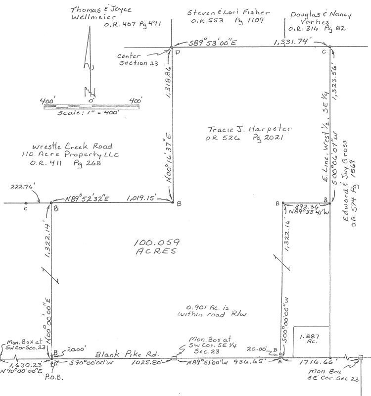
This plat represents a field survey performed in October, 2010. All markers are accurate as to material and location and are in place. All bearings refer to the South line of the Southwest quarter of Section 23 as being N 90° 00' 00" E
