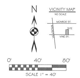
BASIS OF BEARING: BEARINGS ARE OHIO STATE PLANE NORTH ZONE, 3401, NAD 83, GRID DISTANCES SHOWN ARE GROUND.
