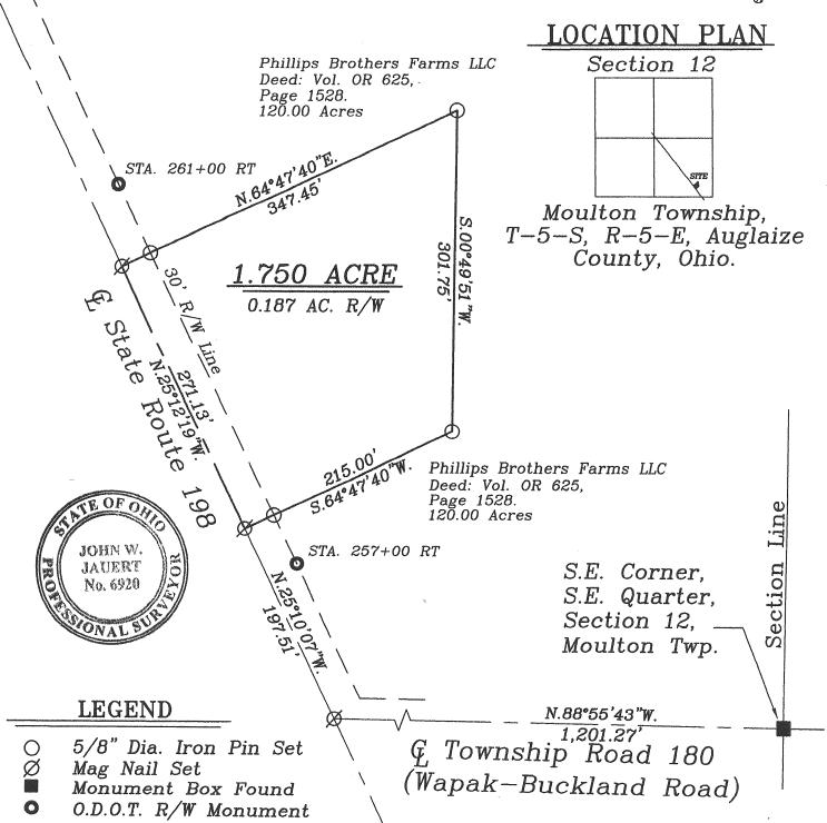
Basis of Bearing is the South Line of the Southeast Quarter of Section 12 and the Centerline of Township Road 180 as N.88°55'43"W. from Auglaize County GPS Survey
