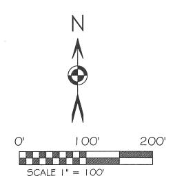
BASIS OF BEARING: BEARINGS ARE BASED OHIO STATE PLANE GRID COORDINATES, NORTH ZONE 3401, NAD 83. DISTANCES SHOWN ARE U.S. SURVEY FEET, GROUND.
