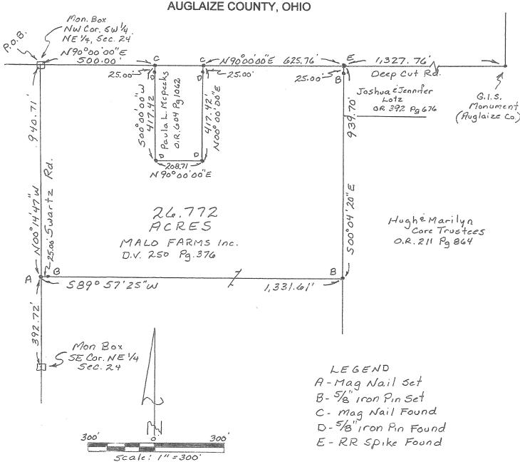
This plat represents a field survey performed in April, 2014. All bearings refer to the centerline of Deep Cut Road as being N 90° 00' 00" E
