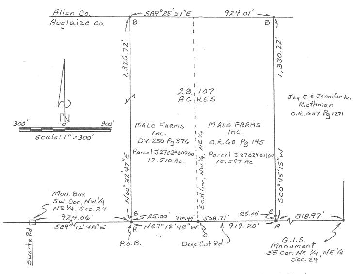
This plat represents a field survey performed in April, 2014. All bearings refer to the centerline of Deep Cut Road as being N 89° 12' 48" W
