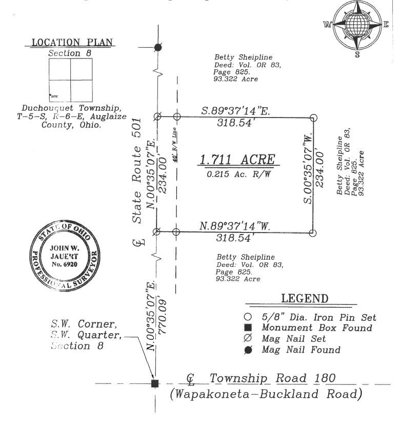
Basis of Bearing is holding the centerline of State Route 501 as N.00 35'07"E. per the Auglaize County Global Positioning Survey.
