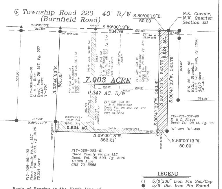
Basis of Bearing is the North Line of the Northwest Quarter of Section 28 Logan Township and the centerline of Township Road 220 as S.88°00'13"E. from the Auglaize County Global Positioning Survey.
