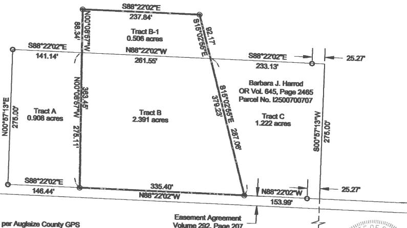
Basis of bearings is per Auglaize County GPS depicting the south line of the northeast quarter of Section 7 as N 89° 09' 12" W.
