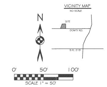
BASIS OF BEARING: BEARINGS ARE OHIO STATE PLANE NORTH ZONE, 340 I, NAD 83, GRID. DISTANCES SHOWN ARE GROUND.
