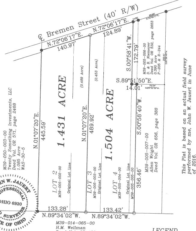
This Plat is Recorded in Survey Book "S", Page 441, in the Auglaize County Engineer's Office. Basis of bearing for this survey is holding the South right-of-way line of Bremen Street and the North line of Lots No. 2, 3, 4 & 5 of the Ernst Eschmeyer's Subdivision as S.72°06'17"W. from previous survey R-244.
