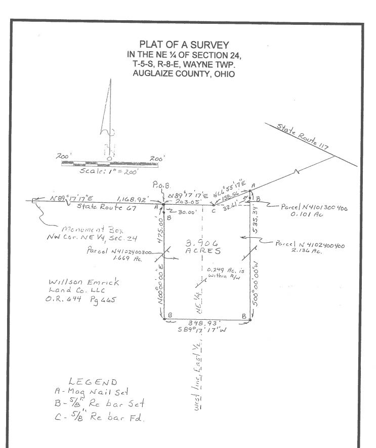
This plat represents a field survey performed in July, 2016. All bearings refer to the north line of the northeast quarter of Section 24 as being N 89° 17′ 17" E
