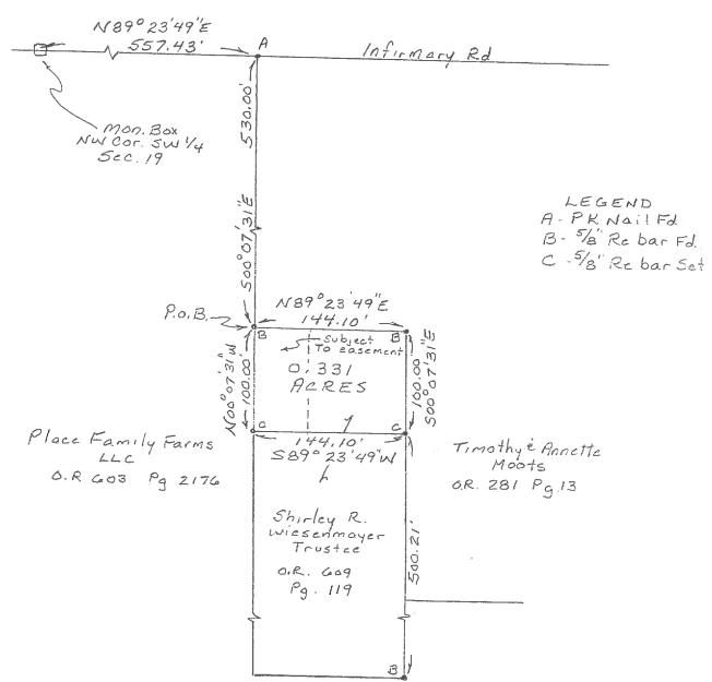
This plat represents a field survey performed in October, 2016. All bearings refer to the centerline of Infirmary Road as being N 89° 23' 49" E
