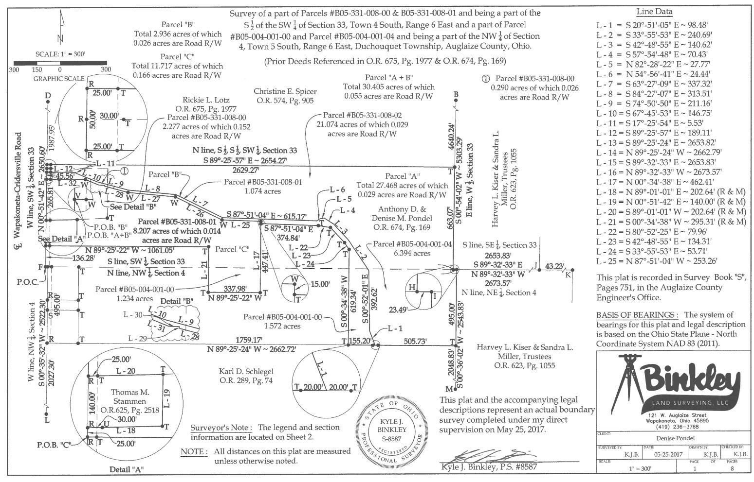
Survey of a part of Parcels #B05-331-008-00 & B05-331-008-01 and being a part of the  $S\frac{1}{2}$  of the SW  $\frac{1}{4}$  of Section 33, Town 4 South, Range 6 East and a part of Parcel #B05-004-001-00 and Parcel #B05-004-001-04 and being a part of the NW  $\frac{1}{4}$  of Section 4, Town 5 South, Range 6 East, Duchouquet Township, Auglaize County, Ohio.
