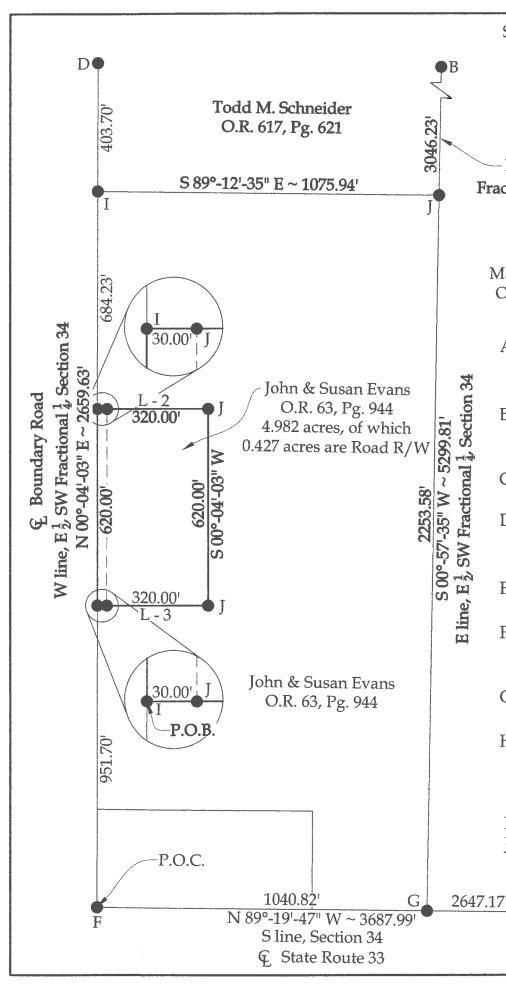
Survey of part of Parcel #L33-034-007-01 and being located in the  $E^{\frac{1}{2}}$  of the SW Fractional  $\frac{1}{4}$  of Section 34, Town 5 South, Range 7 East, Union Township, Auglaize County, Ohio.
