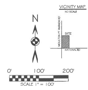
BASIS OF BEARING: BEARINGS ARE BASED UPON THE OHIO DEPARTMENT OF TRANSPORTATION V.R.S., NAD 83(20 | I ADJ.).
