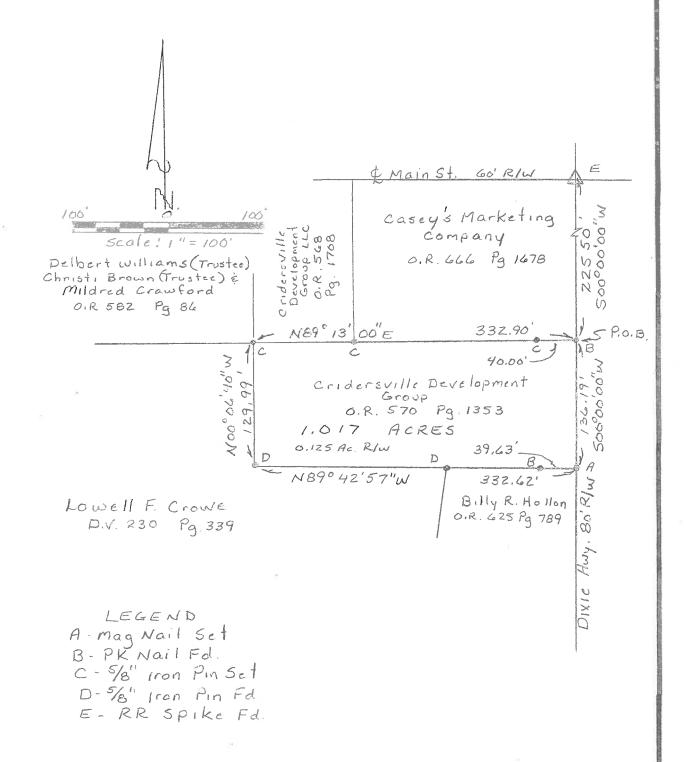
This plat represents a field survey performed in January, 2018. All bearings refer to the centerline of Dixie Highway as being N 00 $^{\circ}$  00 $^{\circ}$  00 $^{\circ}$  E
