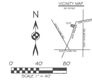
BASIS OF BEARING: BEARINGS ARE ON THE OHIO DEPARTMENT OF TRANSPORTATION V.R.S., OHIO STATE PLANE NORTH ZONE, 3401, NAD 83(2011ADJ.)
