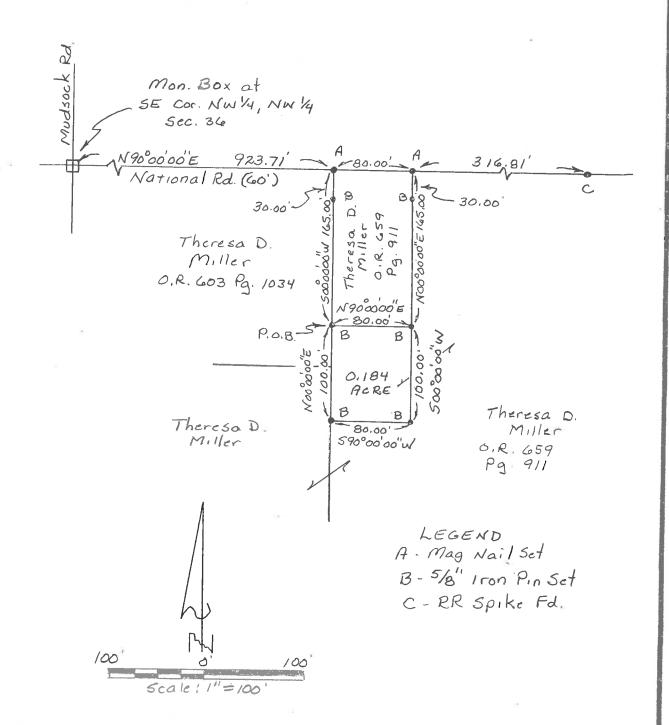
This plat represents a field survey performed in May, 2018. All bearings refer to the centerline of National Road as being N  $90^\circ~00'~00''$  E
