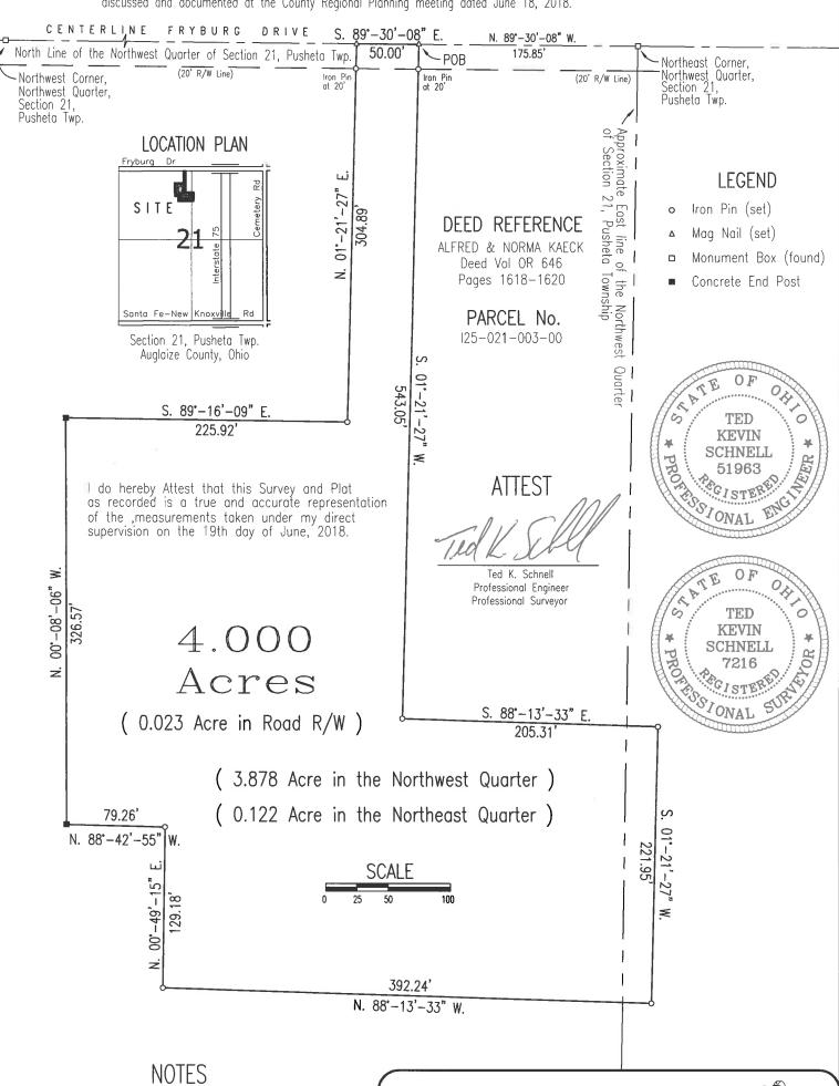
The bearings used for this Survey were determined from the Auglaize County Engineer's Global Positioning Survey and Coordinate System.
