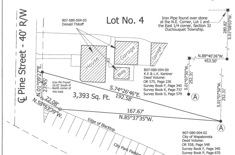
Basis of Bearing is the centerline of Pine Street as N.01009'27"E. based on Ohio State Plane-North Coordinate System NAD83.
