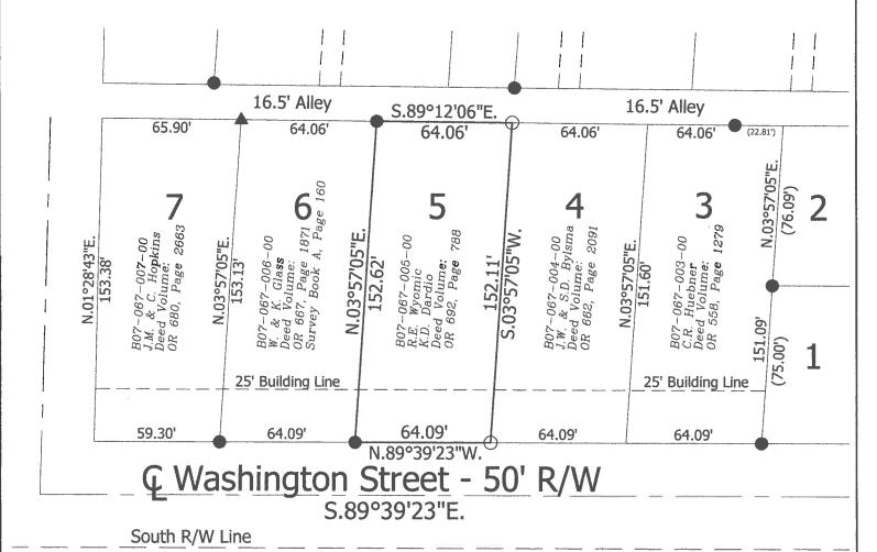
Basis of Bearing is the centerline of Washington Street as S.89°39'23"E. based on the Ohio State Plane-North Coordinate System NAD83.
