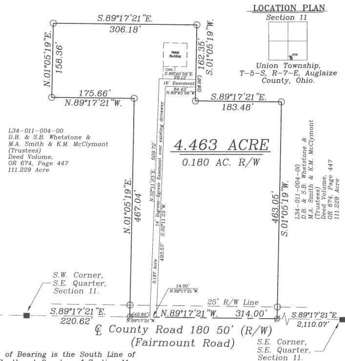
Basis of Bearing is the South Line of the Southeast Quarter of Section 11, Union Township and the centerline of County Road 180 as S.89°17'21"E. from the Ohio State Plane-North Coodinate System NAD83 (2011).
