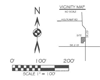
BASIS OF BEARING: BEARINGS ARE BASED ON THE OHIO DEPARTMENT OF TRANSPORTATION V.R.S., OHIO STATE PLANE, NORTH ZONE 3401. NAD 83(2011 ADJ.)
