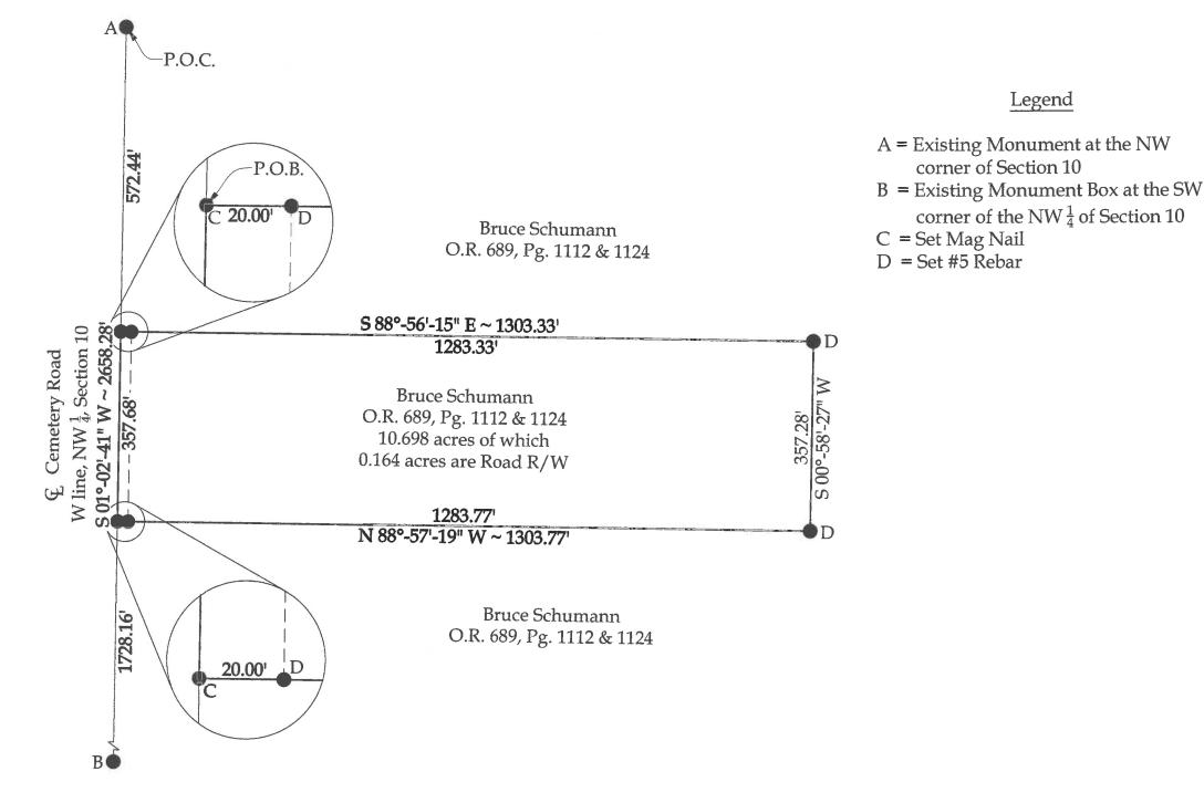
BASIS OF BEARINGS: The system of bearings for this plat and legal description is based on the Ohio State Plane - North Coordinate System NAD83 (2011). This plat is recorded in Survey Book "T", Page 558, in the Auglaize County Engineer's Office.
