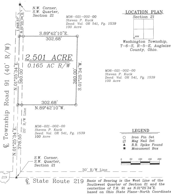
centerline of T.R. 91 as N.01°25'34"E. based on Ohio State Plane-North Coordinate Coordinate System NAD-83 (2011).
